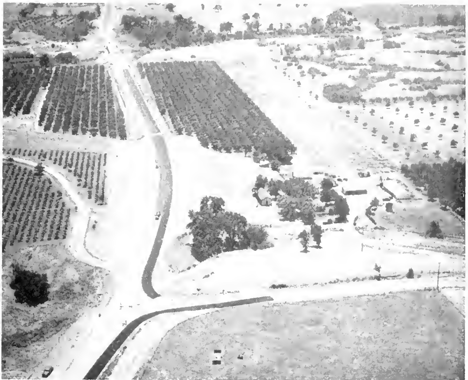
View, south, showing new alignment of Route 97 across Makelumne River and elimination of sharp turn in existing state highway
